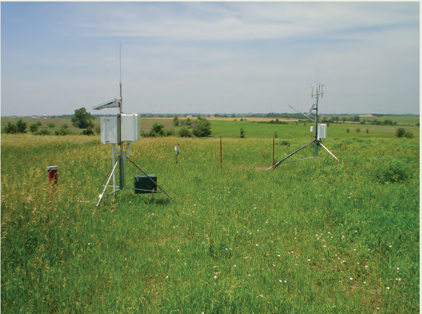
Unsaturated zone equipment and weather station used to study groundwater recharge near Firth, Nebraska.
