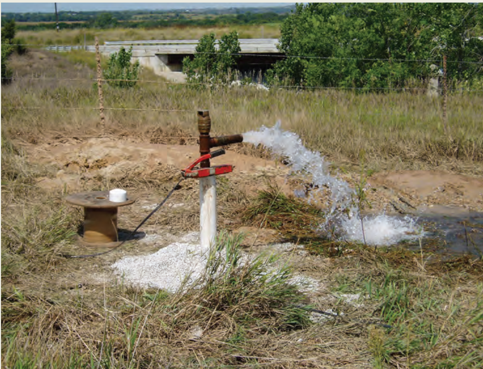
Test well pumps water from Dakota Formation, a secondary aquifer in eastern Nebraska.
