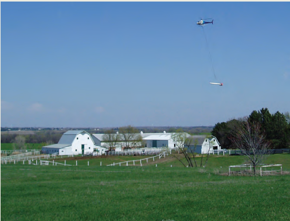
Helicopter electromagnetic survey being conducted in eastern Nebraska.
