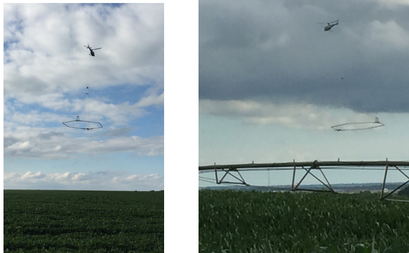
Figure 4-4: Photos of the SkyTEM304M system in suspension beneath the helicopter.
