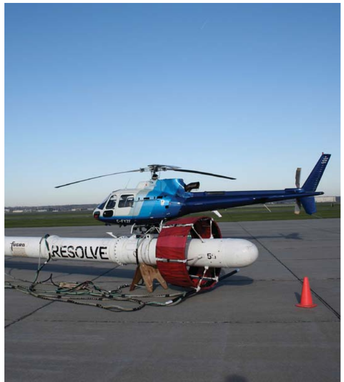
Helicopter used to fly the HEM survey shown behind the cylindrical tube containing electromagnetic hardware.
