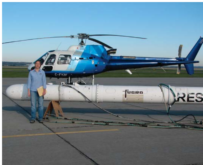
The electromagnetic hardware is encased in a cylindrical tube also called a "bird".
