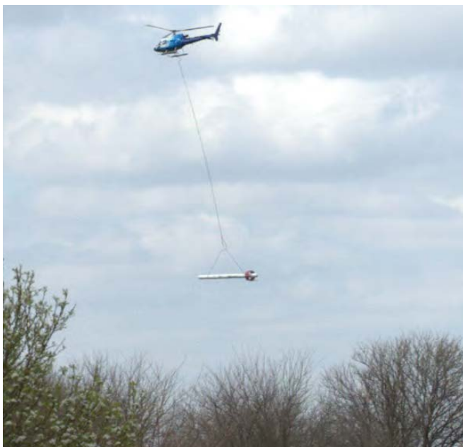
HEM survey being flown over a pasture in the Sprague study area.
