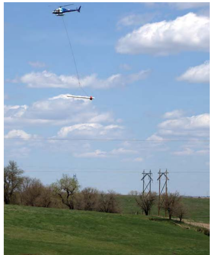
HEM survey being flown over a pasture in the Sprague study area.
