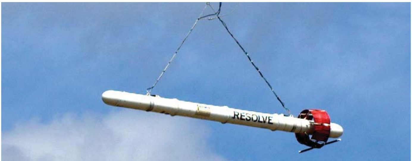
The electromagnetic hardware is encased in a cylindrical tube also called a “bird”.
